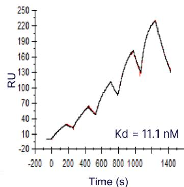
Binding of soluble GPC3 extracellular domain to immobilized ZW251 mAb measured by surface plasmon resonance (SPR)
