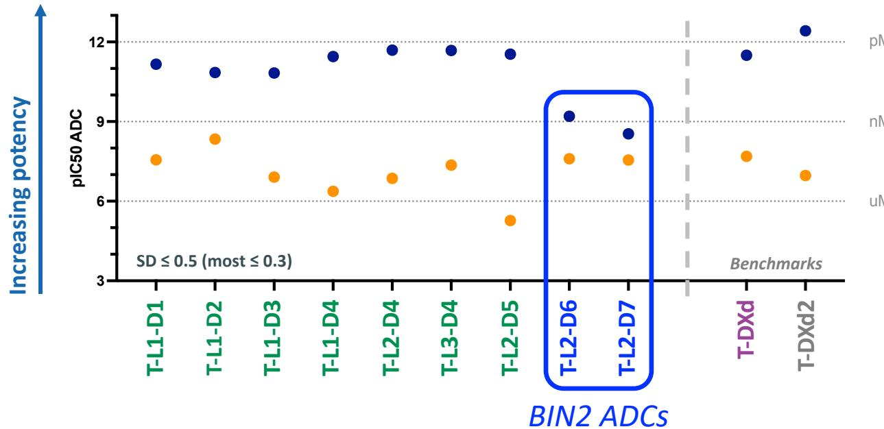
Representative pIC<sub>50</sub> in an Ag+ cell line sensitive to TOPO1i ADCs and an Ag- cell line
